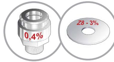
Calibrated orifices are supplied as standard and allow a precise foam concentrate percentage while having a non-return valve function. The suction percentages are: 0,4%, 1%, 3% or 6% depending on your requirement.
