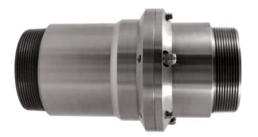
**General** Marine Breakaway coupling Coupling Type Application Mounted between two flexible hoses Nominal Size (Inch) 2 3 5 Min (°C) -50 **Design Temperature** Max (°C) +200 0 0 Min (bar) 0 0 0 Design Pressure Max (bar) 40 40 30 27 23 Maximum flow at activation 50 150 225 100 300 (m<sup>3</sup>/hr of water at ambient temp)
