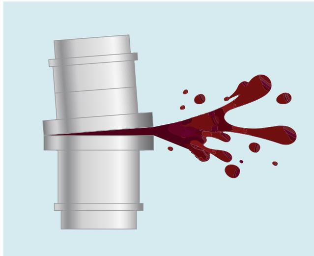
Other Breakaway Couplings can result in uncontrolled spillage in the event of a partial separation.
