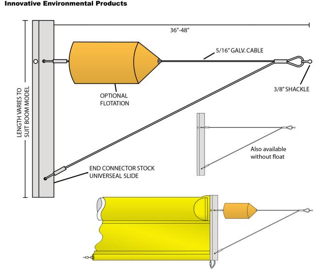
Tow Bridles can be provided with or without auxiliary floats. They may be used for handling the containment boom or silt curtain in water. Prior to deployment, the connector on the tow bridle should be mated to the boom or silt curtain and secured with a toggle pin. The shackle on the tow bridle will accept a line up to 3/4" in diameter. A choice of connectors are available.
